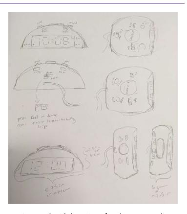
I experimented with locations for these controls as well as the controls I didn't focus on improving (the Time and Alarm Set buttons, and the snooze button). I also experimented with the overall shape of the clock, including a rounded shape to echo the shape of the thumbwheels.
