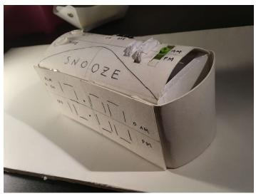
Some users thought that the alarm and time set buttons were onetouch rather than press and hold, due to being raised from the surface. I had left the alarm and time set buttons as press and hold intentionally to prevent users from accidentally hitting the button and changing the time or alarm, so I needed to communicate that interaction better through the buttons' perceptual affordance.
